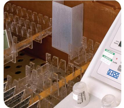
To conduct accelerated corrosion testing in the laboratory, a Q-Fog machine exposes panels to a cyclic environment of salt-laden fog, heat, and humidity.
